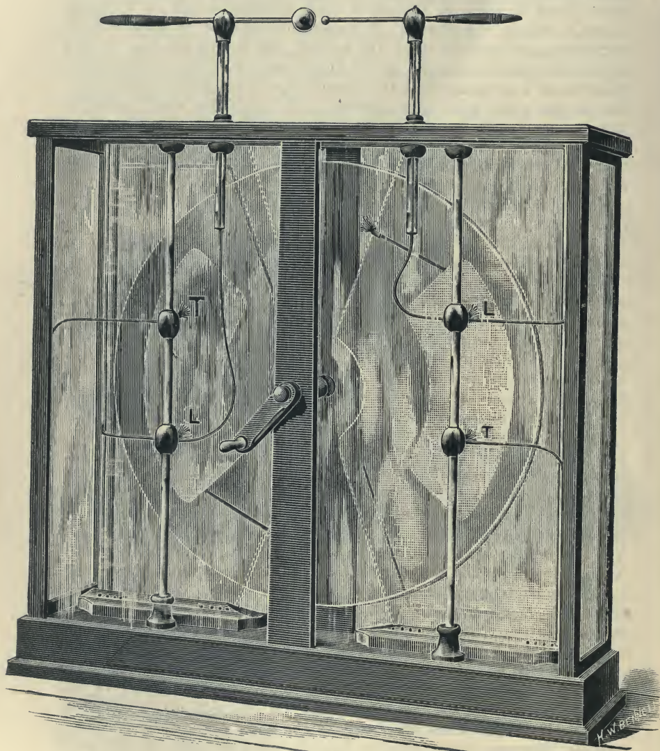
Fig. 92.—Large Wimshurst Machine with Fixed Inductors.
