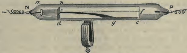
Fig. 682.—Kathode Stream Deflected by a Magnet.
