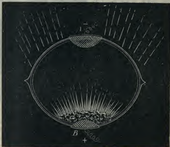
Fig. 678.—Phosphorescence with External Poles.
