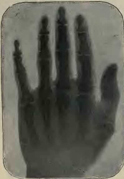
Fig. 696.—Radiograph taken through Black Vulcanised Fibre. (Phot.; Mr. Campbell Swinton.)
