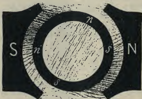
Fig. 480.—Twisted Field as shown by Iron Filings.
