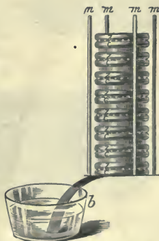
Fig. 130.—Volta's First "Pile."
