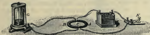
Fig. 384.—Faraday's Discovery of Magneto-Electric Induction.
