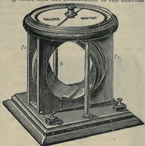
Fig. 776.—Ayrton and Perry's Adjustable Spherical Standard of Inductance.
