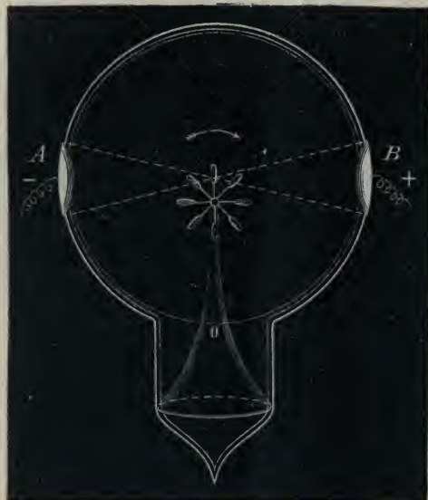
Fig. 680.—Mechanical Motion produced by Radiant Matter. (External Poles.)
