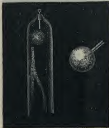
Fig. 671.—Repulsion of Glow by a Conductor.
