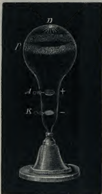
Fig. 675. — Phosphorescence in a Vacuum Tube.
