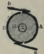
Fig. 545.—Two-part Commutator or Collector.
