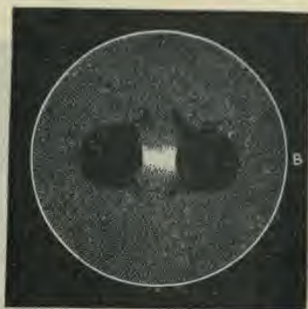
Fig. 51.—Electric Strains between two Charged Cylinders.
